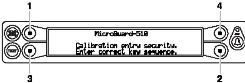
The computer will execute a brief self test and, when finished, enter calibration mode.
