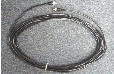
CAN bus from pressure transducer to angle sensor box (see below) PART NO. 10968
