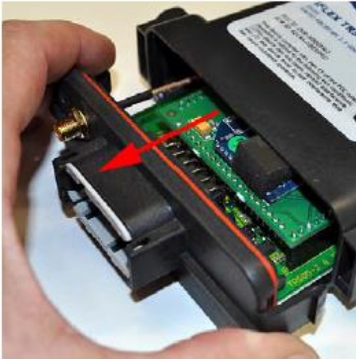
▲ 3. Carefully pull the circuit board out of the housing
