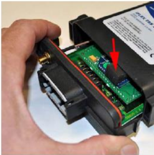
▲ 8. Carefully slide the circuit board into the guide rails in the housing. Make sure that the foam strip is positioned as shown.
