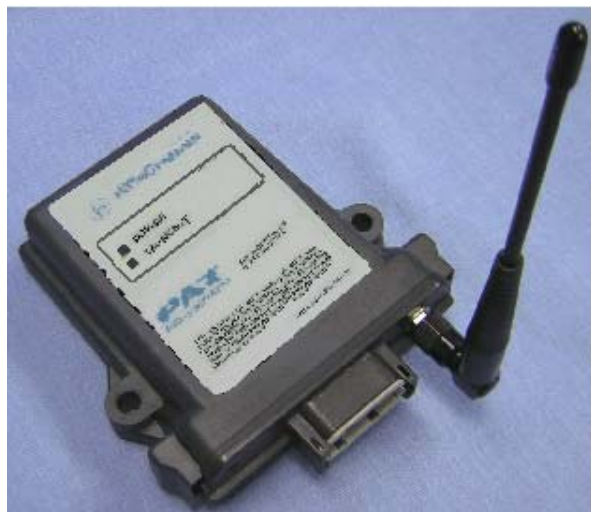
031-300-060-596 TRS 05 REPEATER 031-300-050-688 ANTENNA, 918 MHz RCL 90°
