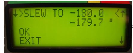
When the console prompts to calibrate certain slew angle points, the unit must be slewed to the appropriate position per instructions depending if the boom rest is forward or to the rear of cab.
