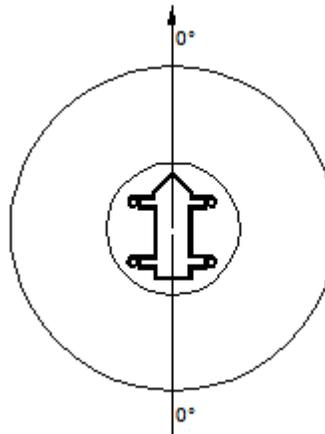
When the console prompts to calibrate certain slew angle points, the unit must be slewed to the appropriate position per instructions depending if the boom rest is forward or to the rear of cab.
