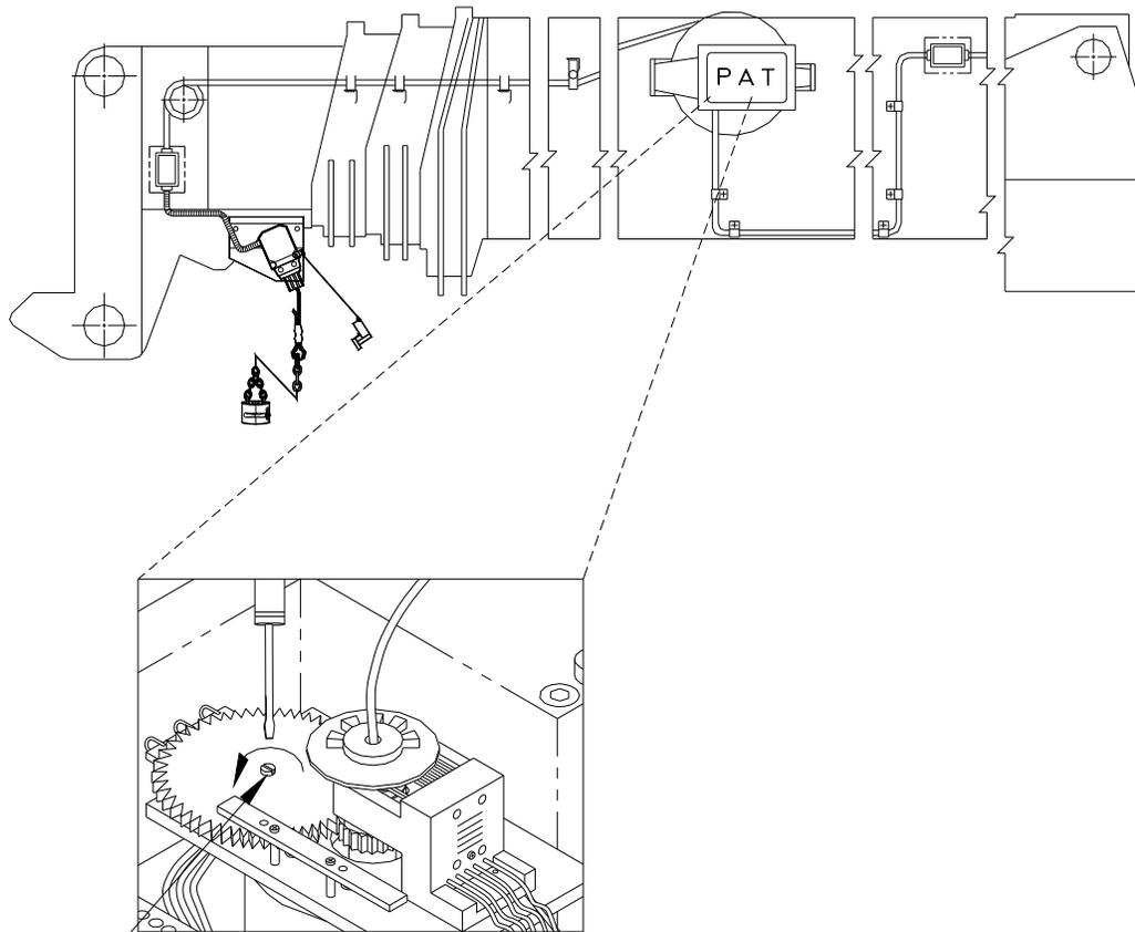
ADJUST LENGTH POTENTIOMETER, WITH BOOM FULLY RETRACTED
