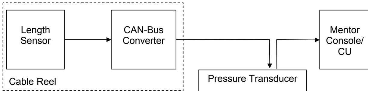
The signal runs from the length sensor to the CAN-Bus converter board, both located in the cable reel. From there, it travels as digital information on the CAN-Bus to the pressure transducer, which acts as a T-connector to the main CAN-Bus running to the console.
