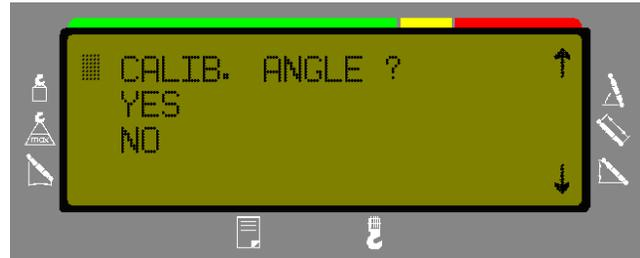
Boom down to a flat angle and mechanically adjust the angle sensor. The angle should be set to +/-0.0 of the measured angle. Material – calibrated inclinometer.
