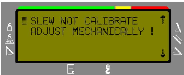
If the slew angle is not within the (+/- 5°) tolerance and 'OK' is selected to confirm the calibration, a screen will be displayed indicating the calibration could not be confirmed and further mechanical adjustment is required.
