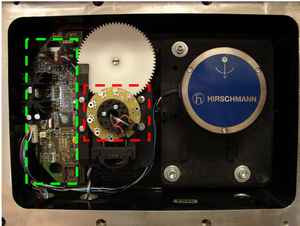
Fully retract the boom and turn the screw of the length potentiometer with a small screwdriver counter clockwise to a soft stop. That should bring the sensor voltage to 0V (+/- 0.1Volt). Measure voltage between Pin 5 (-) and Pin 3 of Terminal X20 and compare.
