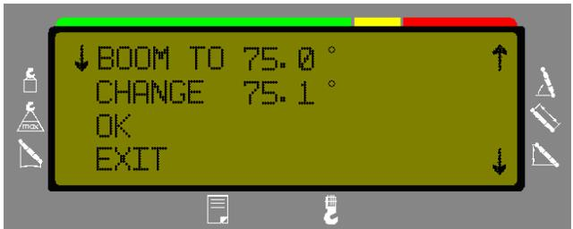
Complete the above procedure to set the correction factor at 40°, 65° and 75° boom angle. After 'OK' is selected the system defines a high boom correction angle, 40°.
