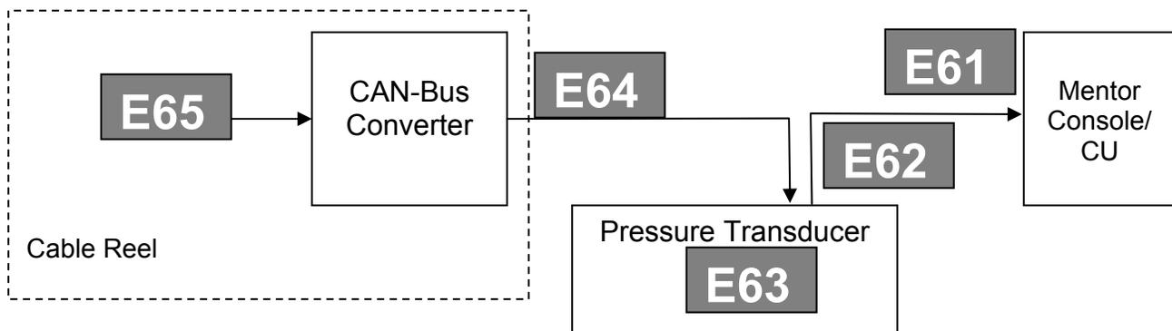
The block diagram tries to clarify that: If the CU does not see any CAN-Bus component, it will report an E61. If it sees only the cable reel, it will report an E62 (pressure transducer missing). If it sees only the pressure transducer, it will report an E64 (cable reel missing). E63 means that the pressure transducer is available, but is reporting an internal error. E65 means that the cable reel unit is available, but is reporting an internal error.
