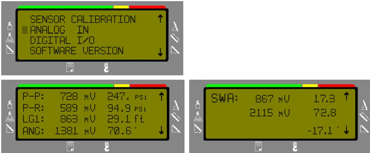
The screen will show all sensor inputs as in the example below. For each sensor, an equivalent voltage is shown in millivolts, along with the physical sensor value that that voltage refers to. Pressure sensors are shown with physical values of [bar], angle sensors and slew sensors in degrees and length sensors in feet (or meters for metric charts).
