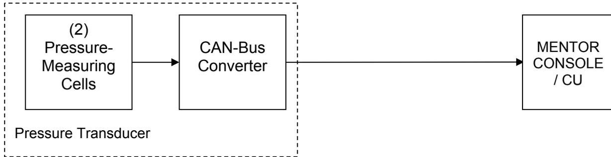
The signal runs from the pressure transducer as digital information on the CAN-Bus to the central unit.
