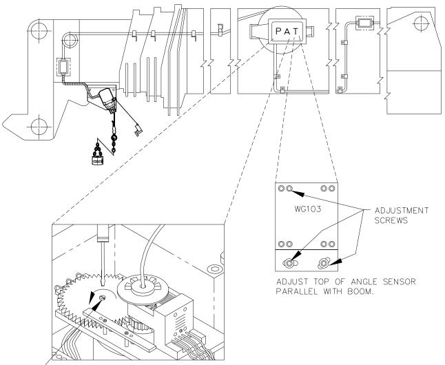
ADJUST LENGTH POTENEIOMETER, WITH BOOM FULLY RETRACTED TURN THE CENTER SCREW COUNTER CLOCKWISE TO A SOFT STOP.
