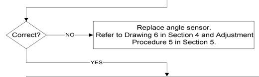
Measure signal from angle transducer in central unit. The return signal is a current output and must be measured in series. Set Voltmeter to measure amps. Remove Wire #4 from X1:4 in the central unit and connect one voltmeter lead to wire #4 and the other lead to X1:4. The measurement should be between 4-20ma. 20ma with the boom at 0° or 4ma with the boom at 90°.
