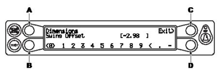
Keys B and D are used to scroll left and right. The "cursor" will appear as flashing < > brackets on either side of the number. Key A is used to enter the number. Key C is used to exit the number entry subroutine.
