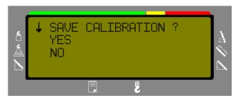
To save the calibration, push the "OK" button after scrolling down to the "Yes" choice.
