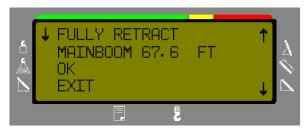
Fully retract the main boom, to continue, press . Press to calibrate. Acknowledge main boom fully retracted.
