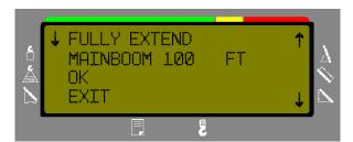
Fully extend the main boom, to continue, press . Press to calibrate. Acknowledge main boom fully extended.
