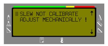
If the slew angle is not within the  $(+/-5^{\circ})$  tolerance and '**OK**' is selected to confirm the calibration, a screen will be displayed indicating the calibration could not be confirmed and further mechanical adjustment is required.
