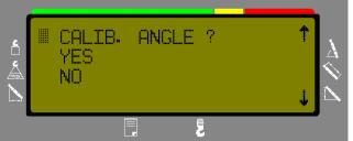
Boom to the slew angle of 0° (+/- 5°) and confirm the calibration by selecting "OK" and then pressing OK. Use the angle to 0°, then press OK. After the display shows the correct radius, press OK.
