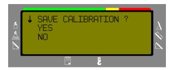
To save the calibration, push the "OK" button after scrolling down to the "Yes" choice.
