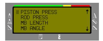
Having successfully entered a valid password, use and keys to mark the piston-side, the rod-side zero setting, and length, and angle calibration. The calibration sensor screen will remain available and accessible without entering the user number until system is power off.
